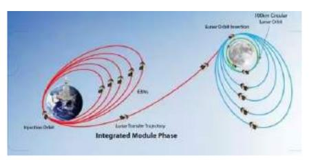
Direct Path vs. Multi-Step Approach: Apollo 11 used a direct trajectory (TLI) to reach the Moon in just over four days, while Chandrayaan-3 follows a multi-step approach, using a series of Earth orbits and engine burns over 40 days to gradually increase speed and position it for lunar insertion.
